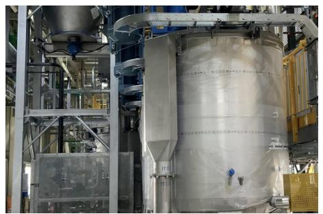
STR stirring units are installed in hot washing modules because thanks to their advanced mechanical action, they improve chemical washing performance and guarantee the best separation of contaminants such as glue and organics while minimising energy, chemical and water consumption.
