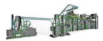
De-inking - ink removal - is an important but underestimated part of the process of recycling. It involves the removal of cured ink systems from a plastic substrate to allow the printed plastic packaging to be recycled and reused in the manufacturing process. This process must be a thorough one, if good-quality recyclate is to be achieved.
