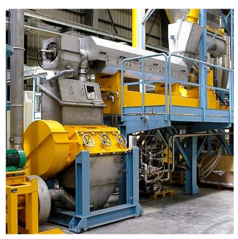
The Key features of TRAMU are the capability to agglomerate the plastics at temperature 20-30% lower than normal extruder and to remove the moisture and the gases at ambient pressure. By operating the machine under the above condition, the TRAMU boasts **the lowest energy consumption**. Easy feeding and wearing have also been strongly controlled while the final density is granted with a calendaring degassing step before the final grinding.
